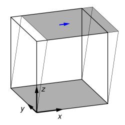
Figure 2.4: dshear test. The upper shaded area represents the rigidly translated boundary surface defined by the shear vector (blue).
