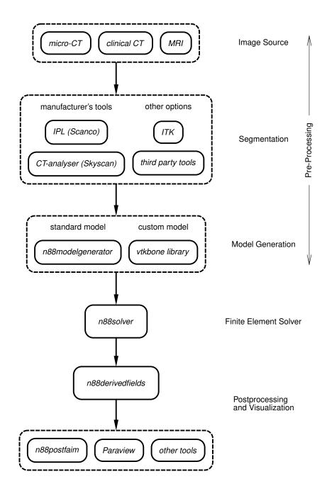
Figure 1.3: Work flow for FE analysis of micro-CT data.
