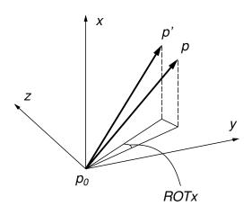
Figure 6.1: Definition of projected angle ROTx.
