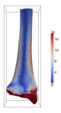
Figure 7.15: Radius in bending test with coloring by von Mises stress
