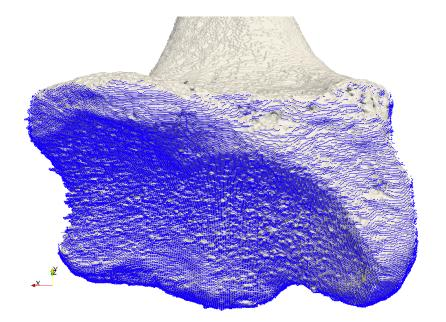
Figure 7.13: Set of nodes on bottom boundary condition for radius bone bending test.
