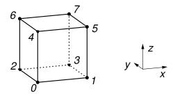
Figure 3.3: Topology of VTK\_VOXEL. Local numbering of the nodes (Points) of the element (Cell) is shown (0-indexed).
