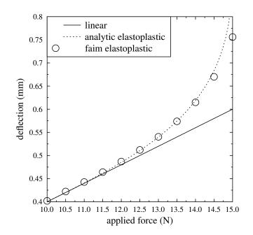
Figure 7.26: Comparison of FAIM and analytic results for elastoplastic cantilever.
