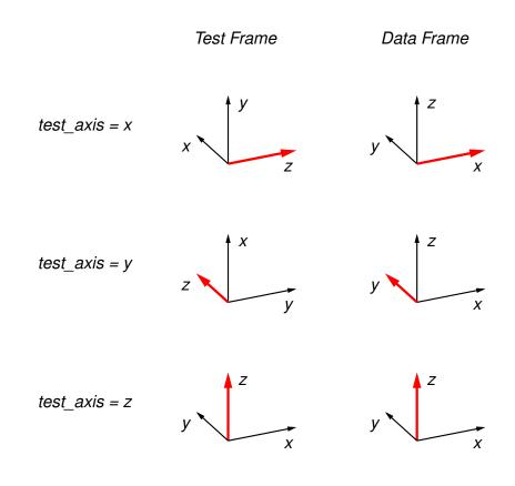
Figure 2.1: Coordinate frames Test Frame and Data Frame as set by the option test\_axis.
