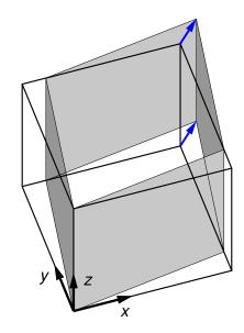
Figure 2.3: symshear test. The side faces (shaded) are displaced as shown.
