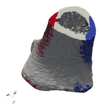
Figure 7.20: A slice through the radius. Yielded elements are shown in red for elements yielded in tension, and in blue for elements yielded in compression.
