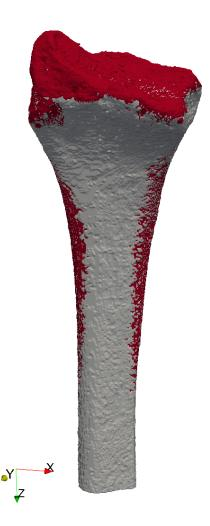
Figure 7.19: Bending radius test with elasto-plastic material properties. Yielded elements are shown in red.
