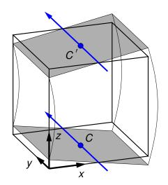
Figure 2.5: Bending test. The shaded areas represent the rigidly rotated boundary surfaces about the neutral axes (in blue). The neutral axes are defined by the central axis (C-C') and an angle in the x-y plane.
