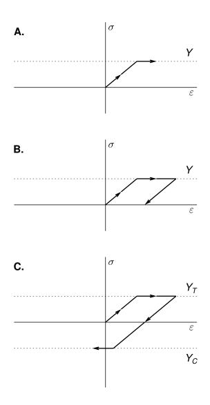
Figure 2.7: Elastoplastic behaviour in one dimension.
