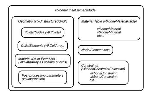
Figure 3.2: Structure of vtkboneFiniteElementModel.
