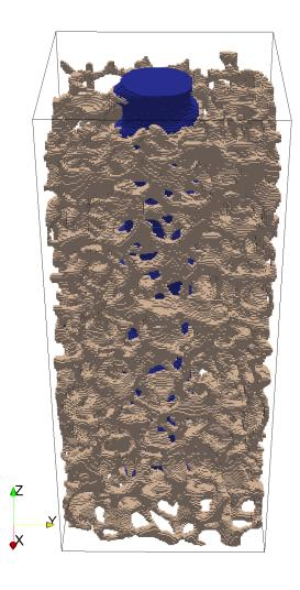
Figure 7.28: Screw model segmented image
