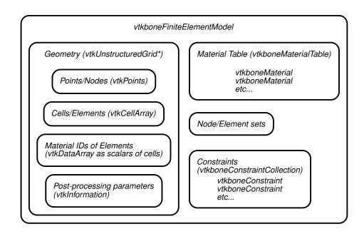
Figure 3.2: Structure of vtkboneFiniteElementModel.
