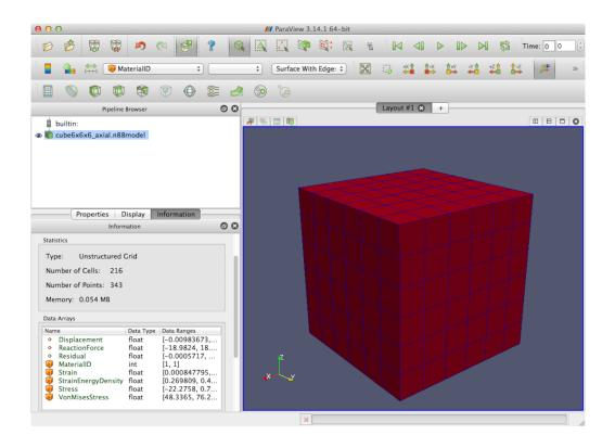
Figure 7.3: Solved 6x6x6 cube with Data Arrays.
