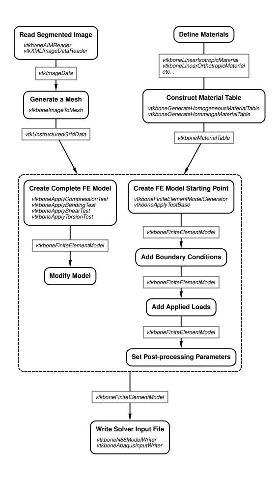
Figure 3.1: Typical work flow for vtkbone.
