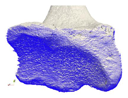
Figure 7.13: Set of nodes on bottom boundary condition for radius bone bending test.
