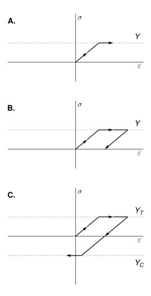
Figure 2.7: Elastoplastic behaviour in one dimension.
