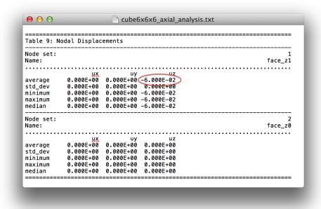
Figure 7.6: uz components in Nodal Displacements table of the analysis file.
