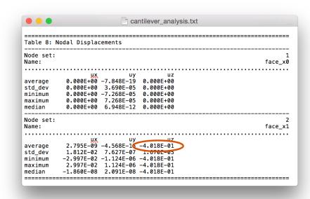
Figure 7.24: Amount of deflection of the end face of the cantilever beam, as found in the analysis file.
