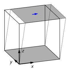
Figure 2.4: dshear test. The upper shaded area represents the rigidly translated boundary surface defined by the shear vector (blue).
