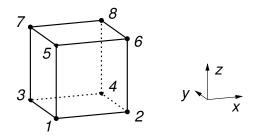
Figure B.1: Topology of hexahedral elements in n88model file (1-indexed).
