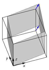
Figure 2.3: symshear test. The side faces (shaded) are displaced as shown.
