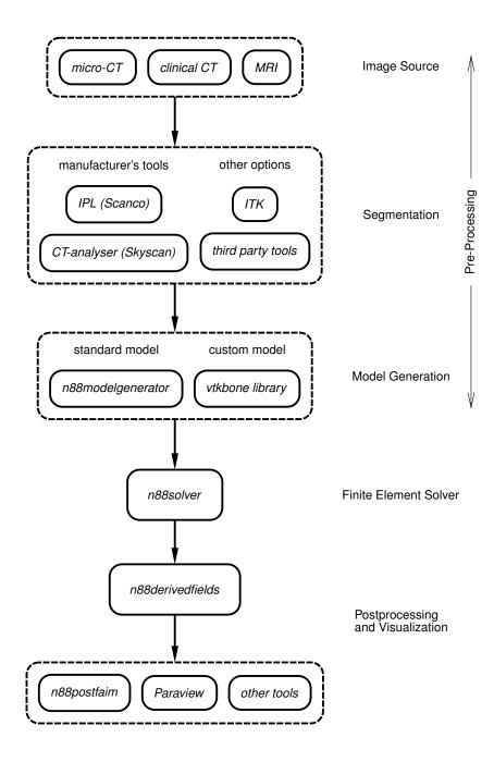
Figure 1.3: Work flow for FE analysis of micro-CT data.
