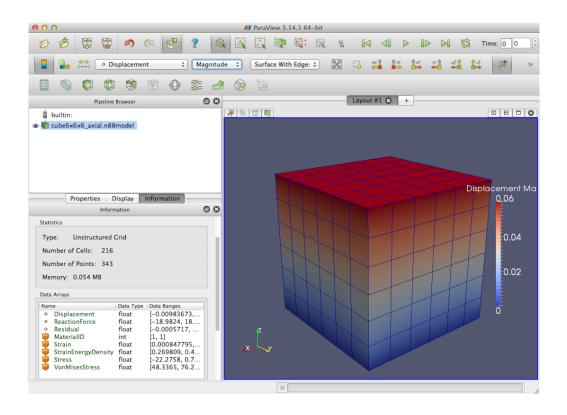
Figure 7.4: Solved 6x6x6 cube colored by Displacement.
